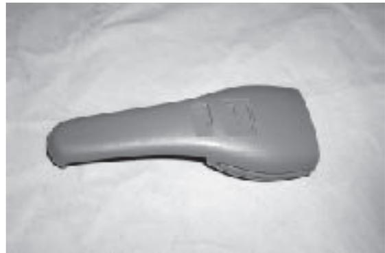
Spray the Stone Gray finish coat next. Two light coats are better than one heavy coat, this may be wet sanded between coats with 600 or finer grit sandpaper if desired.
