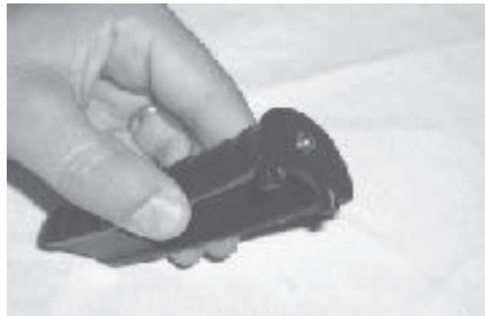
Prepare the emitter by sanding the mold seams and lightly sanding the surfaces. You may keep the impressed window areas present in the raw casting for use as a masking guide later, or sand the whole window ring smooth.
