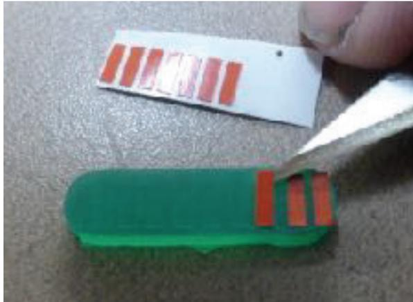
Take your part, and mask the individual LED elements, then spray with gray primer. Spray a coat of clear on it, then when dry peel off the 10 masks, and glue onto your phaser body.
