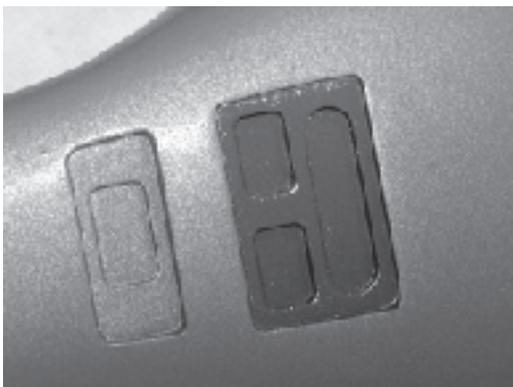
Mask around the top display block with the masking tape and either brush-on or spray a coat of dark gray in the visible area.
