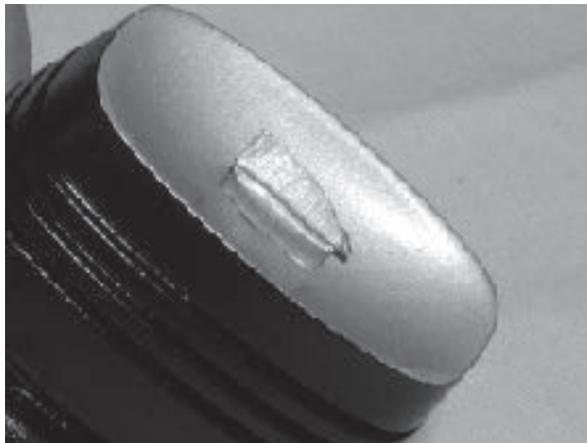
When the paint is cured, mask the emitter so that only the front area is unmasked — leave the tip masking on! Spray this area with light blue metallic — the best one is made by Dupicolor and available in most automotive parts suppliers like Pep Boys or Auto Zone, and the color is a blue-silver.
